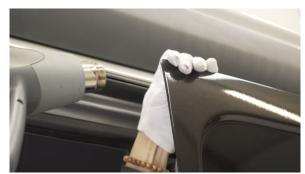
minimise risk of the wrap peeling away at the edges. To post-heat, evenly apply heat across the surface using a heat gun in a smooth motion, heating the surface to at least 90° Celsius. Avoid keeping the heat gun stationary as excessive heat can damage the vinyl. Heat along the edges where the vinyl has been stretched to set it in place.
