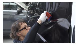
2. Apply Wrap to the Surface Before beginning the application process, perform a final inspection of the surface to make sure that it is thoroughly clean and free from dust and dirt. Begin by peeling away the backing paper and laying the vinyl across the entire surface as flat as possible, avoiding large creases bubbles where possible. Using a
