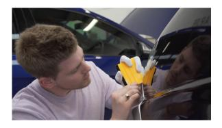
4. Fold and Tuck Edges With your fingers, a squeegee and/or some dedicated tucking tools, fold the excess vinyl around the curved edges of the panel. It is effective to work from the angled corners of the panel into the straighter edges to avoid creases building up under these corners. Use a heat gun to relieve tension and soften the vinyl, allowing it to be stretched around the edge more easily.
